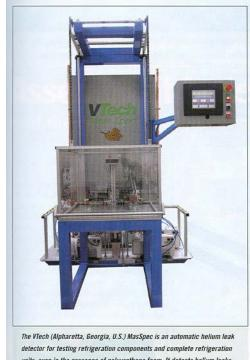
The Viech (Alpharetta, Georgia, U.S.) MasSpec is an automatic helium leak detector for testing retrigeration components and complete refrigeration units, even in the presence of polyurethane foam. It detects helium leaks as small as 0.1 oz of R-134a per year. It requires just 10% helium concentration at atmospheric pressure. Viech is part of Balileo Vacuum Systems
