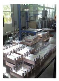
Kaori is currently using the VTech MasSpec for the integral leak detection of their brazed plate heat exchangers. The quality of the leak testing is certified by a calibrated leak and the testing results, thanks to the Data-Logging software accessory, are recorded to a database for data mining and/or print out of testing certificates.
